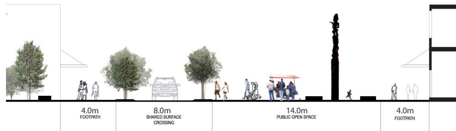
Figure 6. Indicative cross section - corner Jesmond Street and Great South Road - narrowing to one lane and provision of outdoor open space outside the library and southern side of the street
