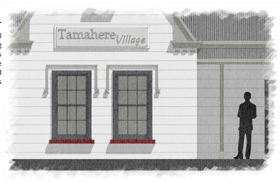
↘ Figure 6. Typical traditional double hung sash windows with decorative mouldings and coloured sills
