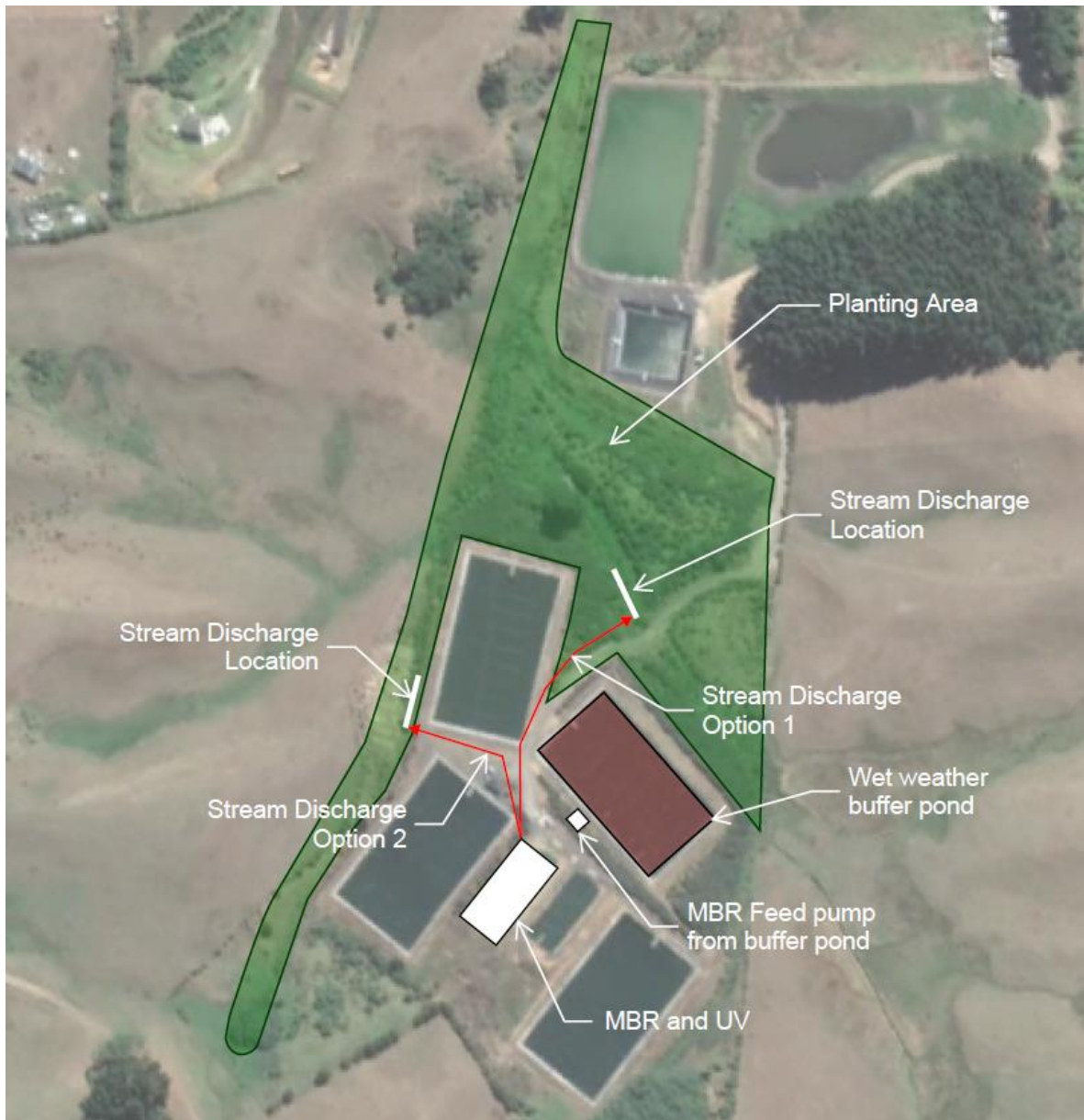
Figure 2 - Proposed MBR and discharge layout
