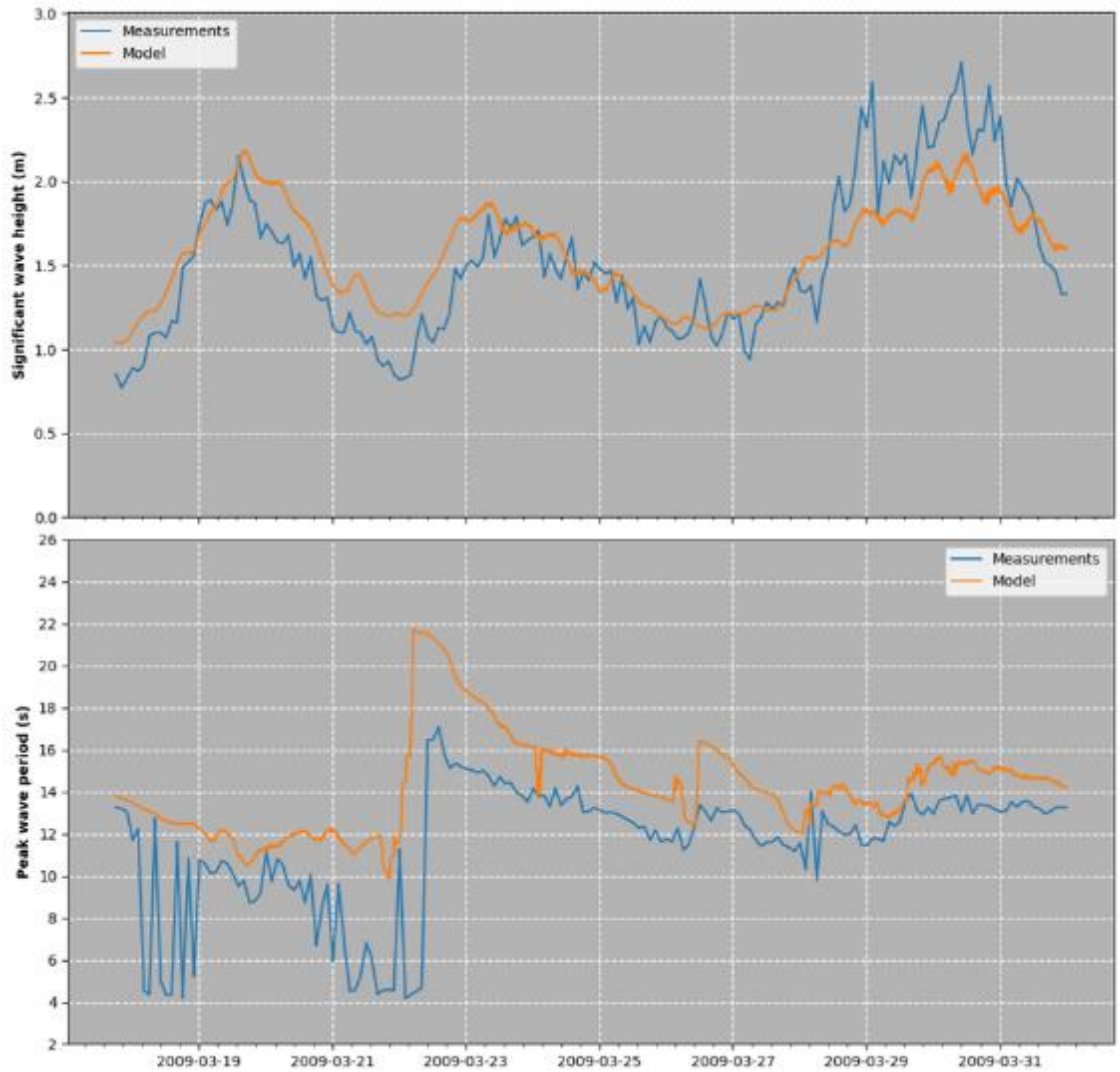
Figure 4-19 Comparisons between measured and model significant wave heights (top panel) and peak wave periods (bottom panels) at Position WB from 18/03/2009 to 01/04/2009.
