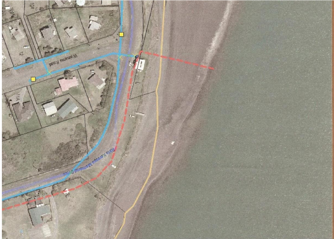
Figure 3-5. Location of the existing pipeline (dashed red line) and discharge point (Diver Services Limited 2009)
