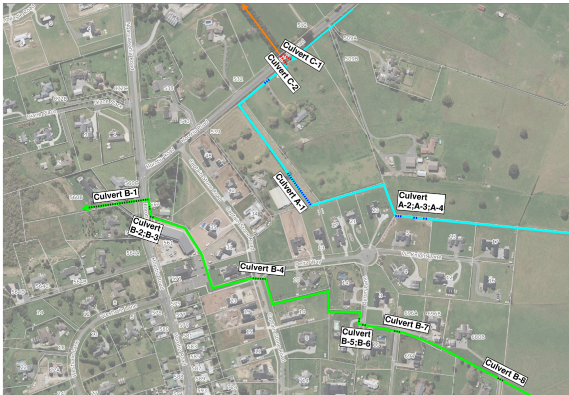
Figure 2 : Existing Culverts along WRC drains
